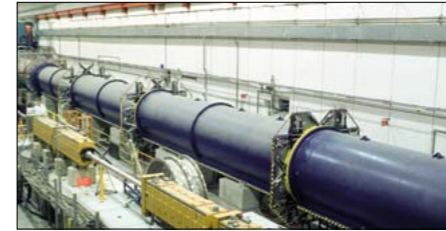
The NA48 experiment at CERN’s Super Proton Synchrotron, which followed NA31 in the 1990s. From right to left: the target for the production the K_S beam (in the blue frame) followed by the multicoloured final collimator; the almost 120-m-long evacuated decay tube; the liquid krypton calorimeter – new for NA48 and key to detecting the decays to neutral pions. (Image credits, right to left: CERN-EX-9610003-07, CERN-EX-9610003-05, CERN-EX-9610003-04.)
