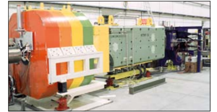
The NA48 experiment at CERN’s Super Proton Synchrotron, which followed NA31 in the 1990s. From right to left: the target for the production the K_S beam (in the blue frame) followed by the multicoloured final collimator; the almost 120-m-long evacuated decay tube; the liquid krypton calorimeter – new for NA48 and key to detecting the decays to neutral pions. (Image credits, right to left: CERN-EX-9610003-07, CERN-EX-9610003-05, CERN-EX-9610003-04.)
