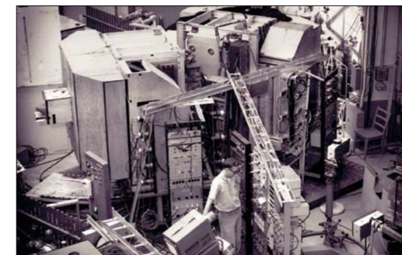
The experiment that discovered CP violation at Brookhaven was set up in a neutral beamline, directed inside the ring of the Alternating Gradient Synchrotron. Visible here are the two spectrometer magnets positioned at 22° to the beam. Spark chambers tracked particles before and after the magnets. (Image credit: Brookhaven National Laboratory.)
