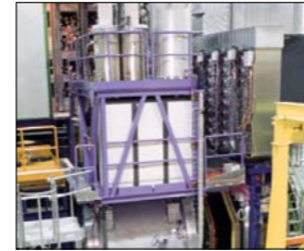
The NA48 experiment at CERN’s Super Proton Synchrotron, which followed NA31 in the 1990s. From right to left: the target for the production the K_S beam (in the blue frame) followed by the multicoloured final collimator; the almost 120-m-long evacuated decay tube; the liquid krypton calorimeter – new for NA48 and key to detecting the decays to neutral pions. (Image credits, right to left: CERN-EX-9610003-07, CERN-EX-9610003-05, CERN-EX-9610003-04.)
